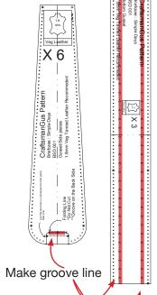
\*\*\* For separate punching method: use guide on the pattern to mark on the gusset and main body pieces to ensure that you have equal amount of holes.
