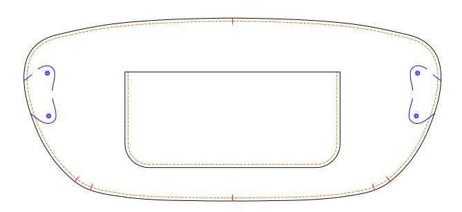
Step 2: Install 180mm zipper on A02, and after that glue A03 on A02 according to the orienting line, also glue and stitch 430mm zipper on. After doing that, you will see a inner pocket is formed between A03 and A02.
