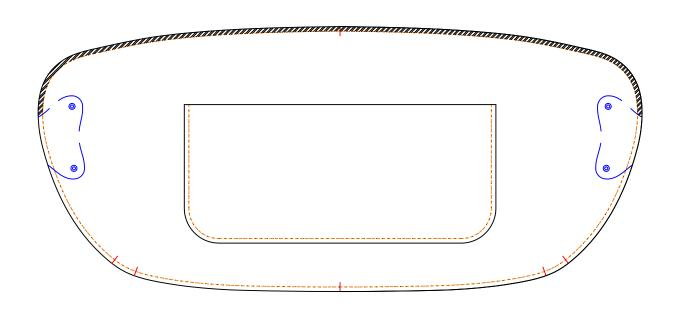
Step 5: Then we only have 2 areas that haven't been glued, please adjust 2 pleats on each side by hand, here we won't say too much, just try, it is easy, after that, you can sew around and install 4 rivets with 2 A05. The bag is OK.
