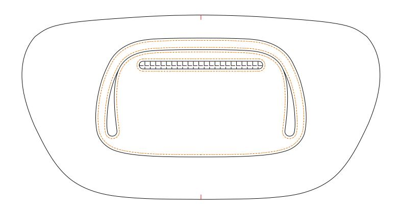
Step 3: The key step is coming. Please paint glue on the edge area that between anchor points, pleat orienting line, and A05's 2 tips. Just glue the downside as sketch shows.
