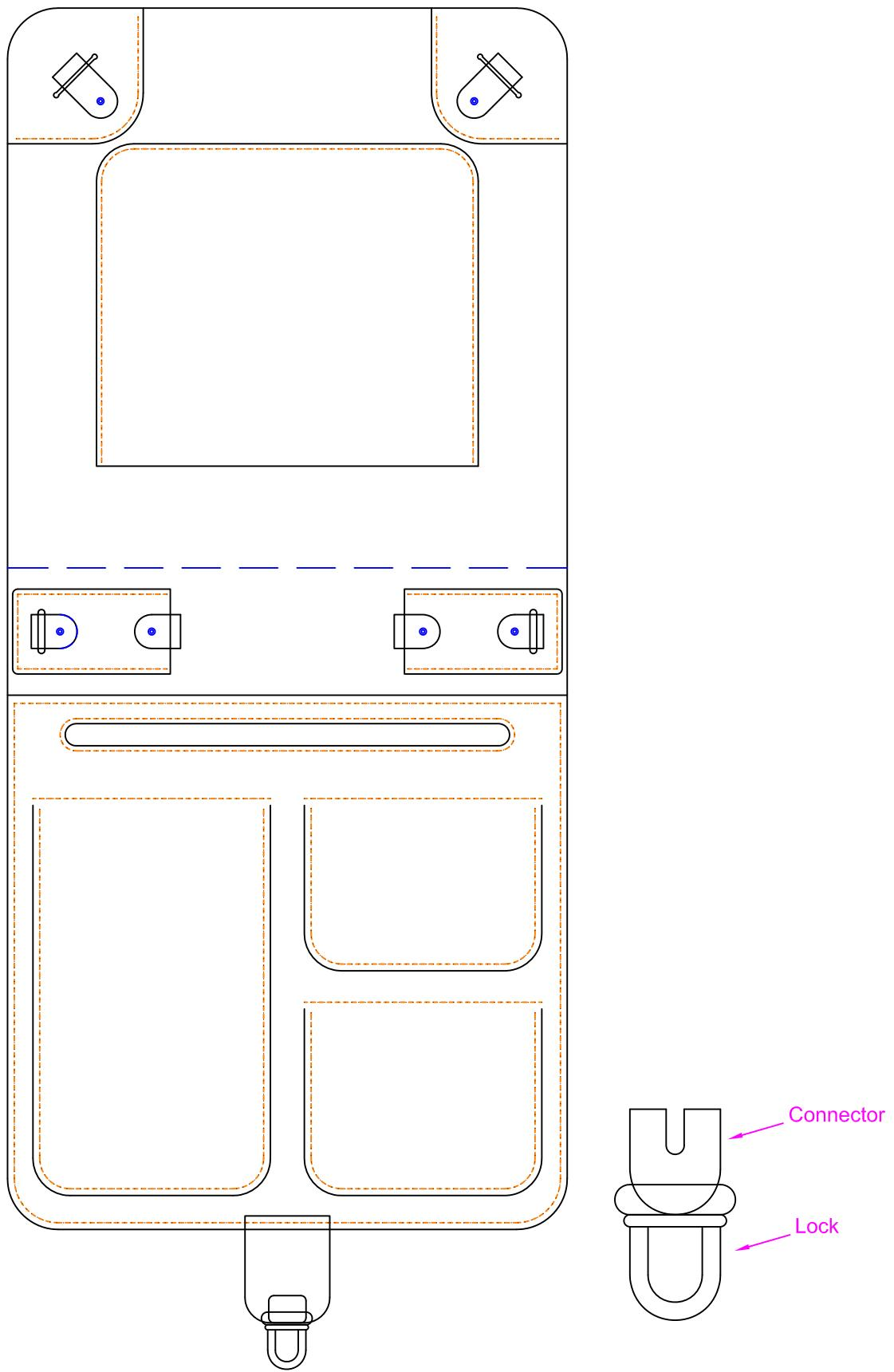
Step 6: Now, we make the handle, the way to make handle is very classic, please learn it carefully. First, fold the handle leather tip to tip by through the D-rings, and then paste the rest part with glue. Second, wrap the wrapper in the middle, and glue firmly. Third, make a stitch in the middle, the handle is OK.
